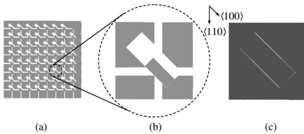
Fig. 3 (a) Mask layouts of the 8 × 8 micro-mirror array. (b) Enlarged view of the mask layout for one mirror and the light-path trenches. (c) Backside mask layout of one cantilever
