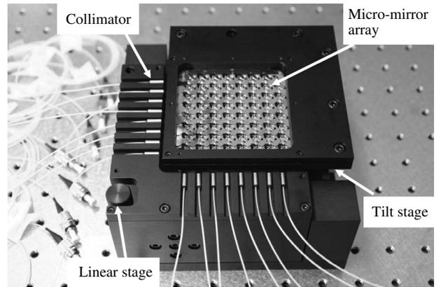
Fig. 6 The prototype of the assembled  $8 \times 8$  optical switch
