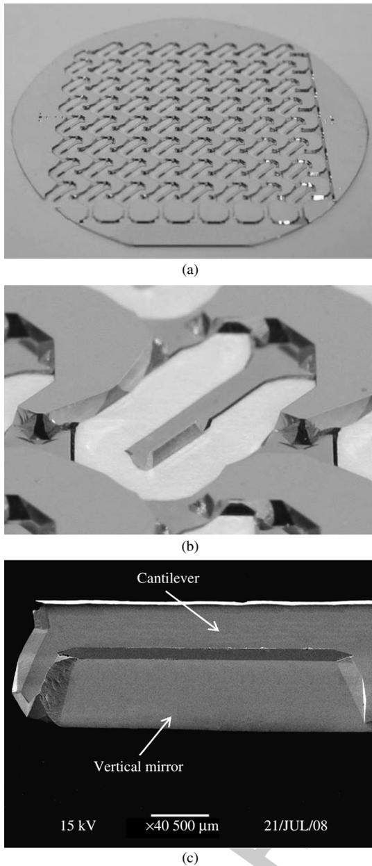
Fig. 5 (a) A picture of the fabricated  $8 \times 8$  micro-mirror array. (b) An enlarged view of a cantilever with a movable mirror. (c) An SEM picture of the vertical mirror and the cantilever
