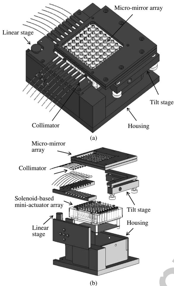
Fig. 1 (a) The schematic drawing of the proposed  $8 \times 8$  optical switch. (b) The corresponding exploded view of the switch
