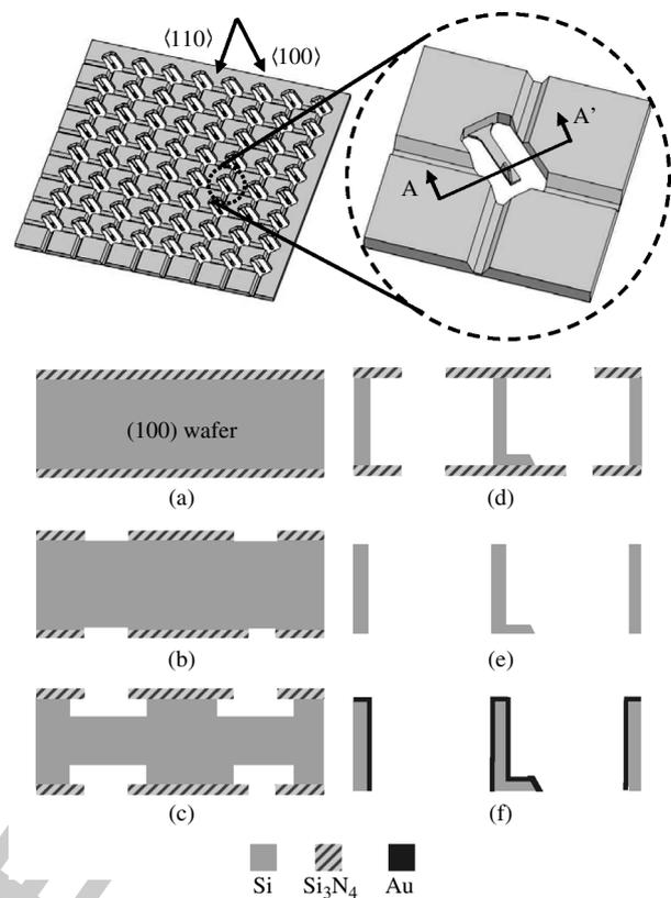
Fig. 4 The fabrication process of the silicon micro-mirror array. (a) The (100) silicon wafer is deposited with silicon nitride layers. (b) Patterns transferred. (c) The beginning of the KOH etching process. (d) The micro-mirror array is created after the KOH etching process. (e) The residual silicon nitride layers are removed. (f) The fabricated micro-mirror array is deposited with gold
