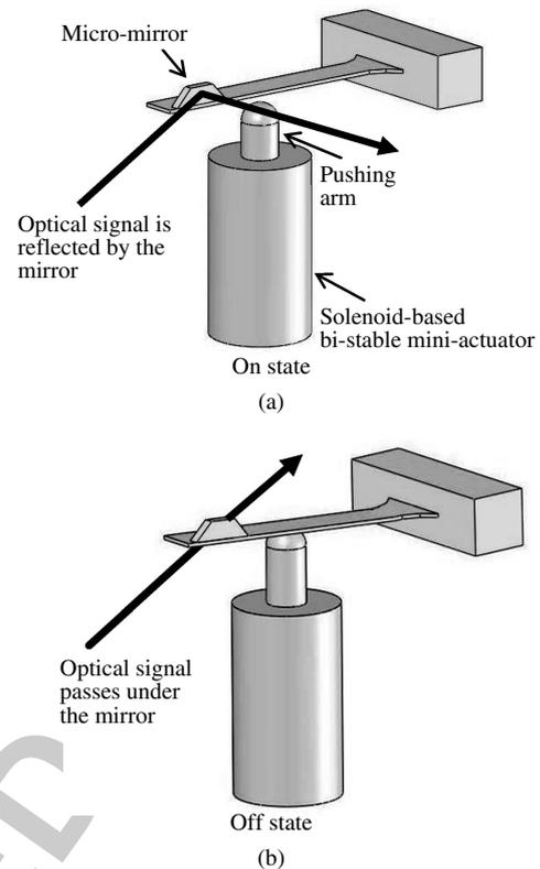
Fig. 2 The operational principle of the switch. (a) On state, the pushing arm does not contact the cantilever such that the micro-mirror can precisely reflect the optical signal. (b) Off state, the cantilever is pushed up by the pushing arm and the optical signal can pass through under the mirror
